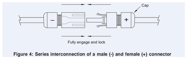
Figure 4: Series interconnection of a male (-) and female (+) connector
