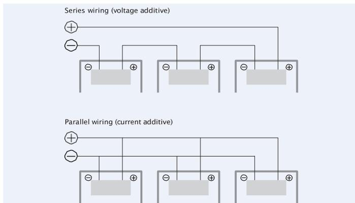
Figure 3: Electrical diagrams of series and parallel wiring
