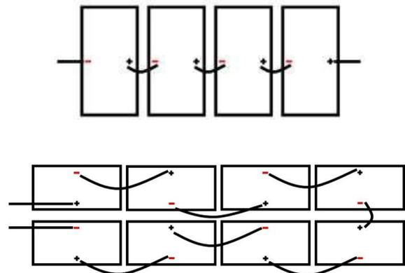
Figure 2: Wire loop design recommendation
