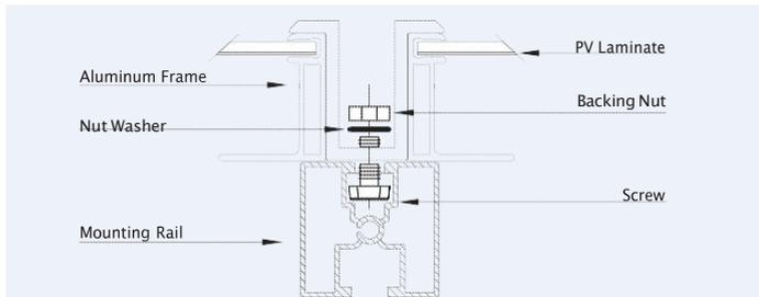
Figure 10: Detail of a top-down clamp mounting attachment
