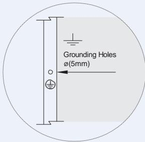
Figure 6: Grounding hole detail
