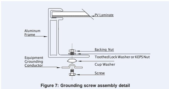
Figure 7: Grounding screw assembly detail
