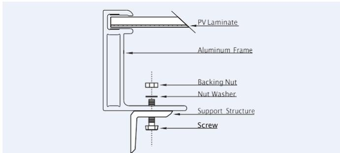
Figure 9: Detail of a bolt mounting attachment
