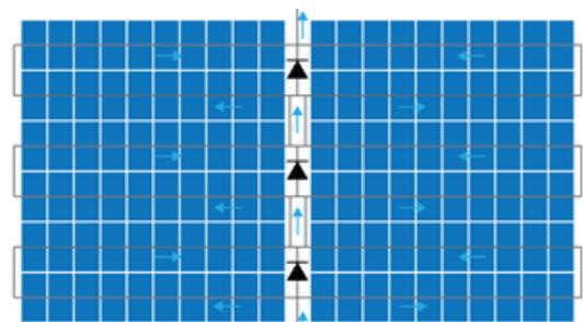
Figure 5: Electrical circuitry of cells and bypass diodes
